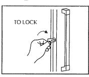
Key pops out for security – store in safe place. To lock or unlock the freezer you must push the key in the lock while turning. The lock is spring loaded so the key cannot be left in the lock.
